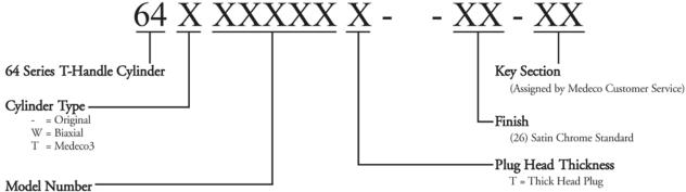
0155 = 5 Pin spring bolt, zinc bolt, zinc shell 0155C = 5 Pin deadbolt, zince bolt, zinc shell 0750E = 4 Pin spring bolt, zince bolt, zinc shell 0750G = 4 Pin deadbolt, zinc bolt, zinc shell 0950 = 4 Pin spring bolt, steel bolt, zinc shell 0952 = 4 Pin deadbolt, steel bolt, zinc shell 1050 = 4 Pin spring bolt, steel bolt, steel shell 1051 = 4 Pin deadbolt, steel bolt, steel shell
