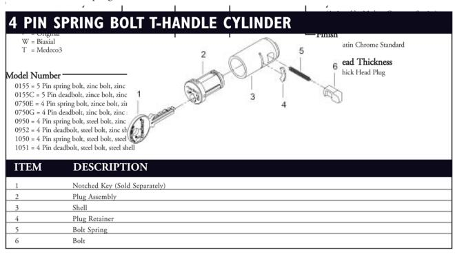
With enhanced security features, Medeco's 0950 series T-handle cylinders are for use in higher risk locations where the chance of physical attack is greater. With a solid steel bolt and reinforced shell, the 0950 is designed to resist would be thieves. Available in a 4 pin body style with either spring or deadbolt functions.
